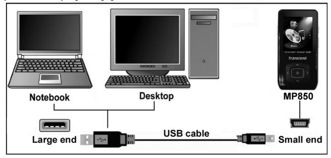
Figure 2: Connecting to a Computer
